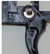
Trigger spring adjusted to 40 Degrees: The leg of the spring will cut through the M of the M-K logo
