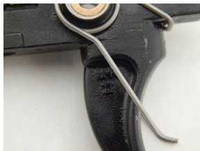
Trigger spring adjusted to 20 Degrees: The leg of the spring will cut through the K of the M-K logo.
