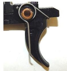
Trigger spring adjusted to 45 Degrees: The leg of the spring will run along the rear edge of the trigger bow
